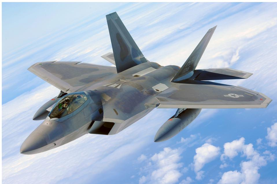
Figure 2.1: Lockheed Martin-Boeing F-22 Raptor. The hole under the cockpit is the intake of an S-duct leading to the engine in the rear part. The hole and the engine are not aligned, so the duct needs to be S-shaped.
