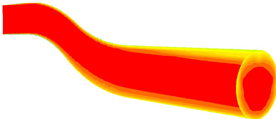
Figure 4.1: Total pressure for the flow on a mesh that does not properly capture the separation phenomenon of the flow. Green is  $1.01 \times 10^5$  Pa and red is  $1.07 \times 10^5$  Pa.
